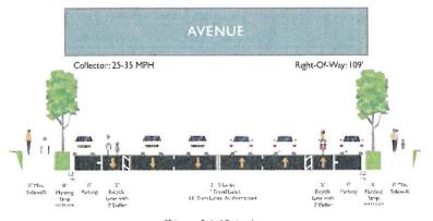
75' between Back-of-Curb sections Includes Parking and Buffered Bicycle Lanes
